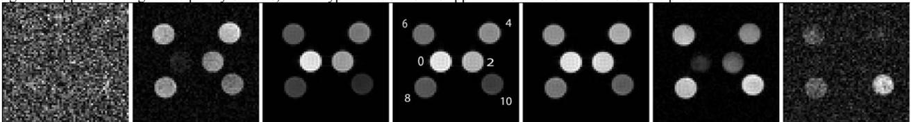
Figure 1. MAVRIC images from the phantom setup for 7 discrete transmission and reception center frequencies, using a bandwidth of 600Hz. From left to right: -600Hz, -400Hz, -200Hz, 0Hz ( $f_0$ ), +200Hz, +400Hz, +600Hz. Images are scaled differently for visualization. Concentrations of HoMS are indicated in the central image in mg/ml.
