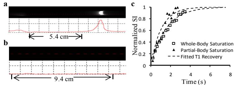
**Figure 1.** (a)&(b) Signal intensity profile along the long axis of the cylindrical water phantom. Partial-body and whole-body saturation was achieved by the mouse coil and rat coil with length of 7.8 and 18 cm, respectively. (c) Normalized signal intensity (SI) evolution of the left ventricular blood after saturation preparation in mouse.
