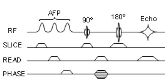
Figure 1. IR-SE pulse sequence using selective AFP inversion pulses for localized volume selection and spin inversion.
