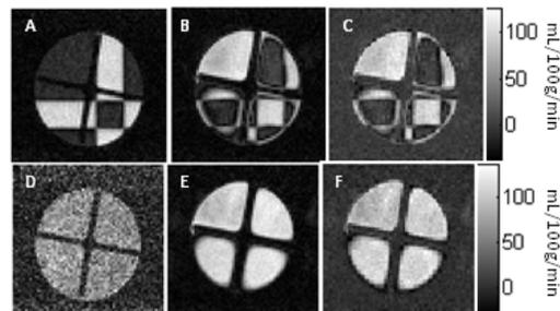
Figure 2.  $T_1$ -weighted images generated using volume-selection IR-SE sequence (A,B) and slice-selection IR-SE sequence (D,E) at flow rates of 0 and 120 mL/min; FAIR images collected with volume- (C) and slice-selection (F) at the flow rate of 120 mL/min.
