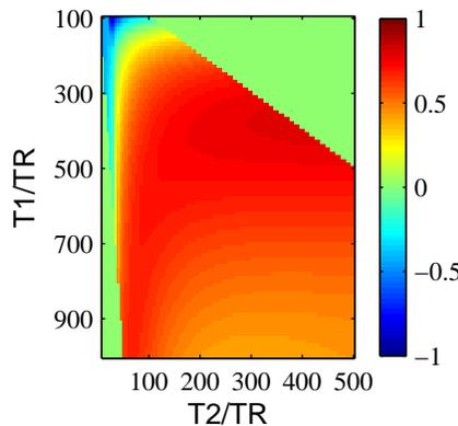
**Fig. 2:** The relative difference (in percent) between  $\alpha$  and the numerically determined  $\Omega$ , for  $0.05 < T2/T1 < 1$  (simulated, without noise). Sequence parameters as in Fig. 1. The first 3 echoes were excluded from the calculation of  $\Omega$  (see text).
