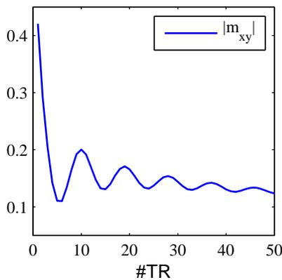
**Fig. 1:** The approach toward dynamic equilibrium is associated with superimposed oscillations. Shown is the simulated magnitude over 50 TR cycles ( $T1/T2/TR = 150/15/1$ ,  $\alpha = 40^\circ$ ), with intermittent idle periods of duration 100.
