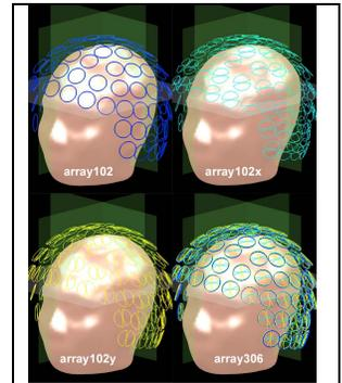
**Figure 1.** The geometries of using 102 or 306 pick-up coils to cover the whole head. Orthogonal slices for *g*-factor calculation are illustrated by translucent planes.
