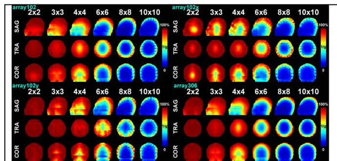
**Figure 2.** The spatial distribution of 1/*g*-factor in mid-sagittal, mid-coronal, and one axial slice using array102, array102x, array102y, and array306 geometries at R=2x2, 3x3, 4x4, 6x6, 8x8, and 10x10 respectively.
