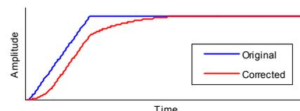
Figure 2 Gradient waveforms calculated from original (blue) and optimal (red). Note that the time constants of the function between the beginning of ramp-up part and the end of ramp-up part were different in the optimal case.
