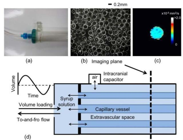
Fig. 1 (a) Lateral view of the phantom, (b) microscopic image of imaging plane, (c) acquired ADC image in a state of rest, and (d) phantom for simulating that the water fluctuation was affected by biomechanical factors.
