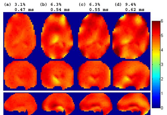
Fig. 5. Simulated FA homogeneity obtained using the  $k_T$ -points technique for performance and robustness analysis: (a) ref. phantom-16 independent channels, (b) ref. phantom-8 ideal modes, (c) ref. phantom-8 synthesized modes, (d) modified phantom-8 synthesized modes.
