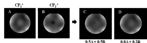
Fig 3: The optimal combination based on weighted images (C / D =  $0.5A + 0.5B / 0.8A + 0.2B$ ) of GRE water sphere phantom images generated by  $CP_1^+$  mode (A) and  $CP_2^+$  mode (B).
