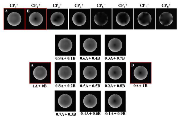
Fig 2: GRE sugar/water phantom. **Top row:** images generated by  $CP_1^+$  mode and clockwise higher CP modes. **Remaining rows:** to estimate the optimal image combination, selected combinations of weighted  $CP_1^+$  mode (A) and  $CP_2^+$  mode (B) were generated.
