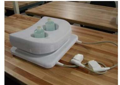
Fig. 3 Picture of the 7T breast array coil
