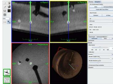
**Fig. 2:** Screenshot of navigation scene. Targets appear hyperintense, model vessels as signal voids. Virtual instrument is overlaid on three orthogonal views. Position was controlled with T1w VIBE scan (TR/TE=3.8/1.7 ms, matrix 256x167, 0.4x0.4x2 mm<sup>3</sup>, TA=22 s).
