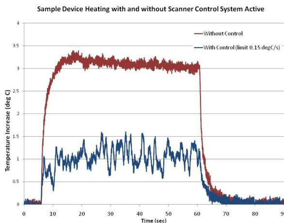
**Figure 2:** Device heating profiles with and without the system active. Enabling the system limited heating by altering the scan parameters according to temperature increase rates.
