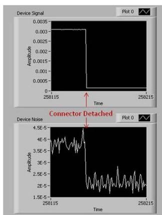
**Figure 1:** Signal and noise plots for the device channel. This demonstrates sudden drop when the device is disconnected and triggers a low-power scan mode.
