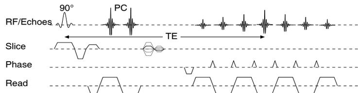
**Fig. 1:** Basic EPI sequence used involving z-shim gradient pulses and flow rephasing in slice direction. “PC” denote the reference scans acquired to correct N/2 ghosts.
