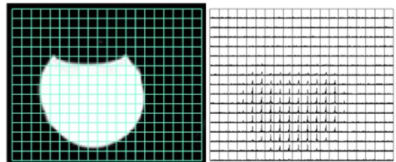
Figure 1: Phantom validation data acquired using the new compressed sensing design. The location of  $^{13}\text{C}$  acetate signal (right) is consistent with a T2 weighted image of the phantom (left).
