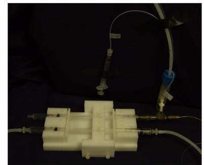
Figure 1: Hydraulically drive automated MR compatible syringe pump.
