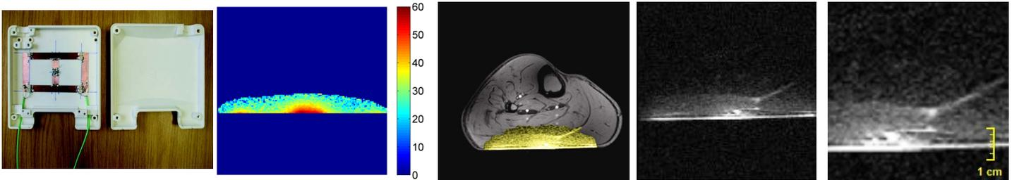
**Fig. 1:** Home built 2 channel capacitively decoupled  $^{23}\text{Na}$  surface loop (5 x 6 cm) coil, based on the design in [3].
