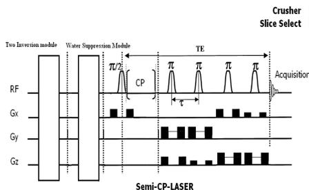
Fig. 1. Semi-LASER sequence diagram
