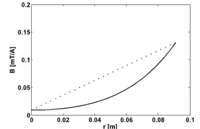
**Figure 1:** Magnetic field of the homemade non-linear (continuous) and a hypothetical linear (dotted) radially symmetric gradient. The latter is non-physical as the derivation of the magnetic field is not continuous at the origin.
