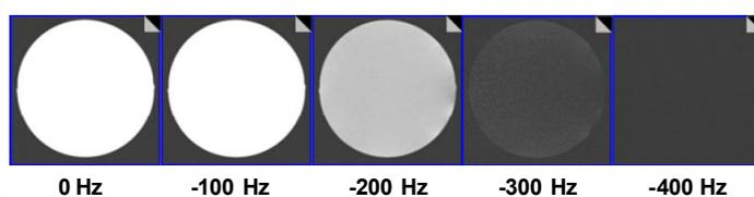
**Fig. 2.** Center slice from 3D-TSE acquisitions of a spherical phantom as a function of off-resonance frequency from 0 to -400 Hz, demonstrating the frequency-selective characteristics of the first refocusing RF pulse. Window/center settings are identical for all images.
