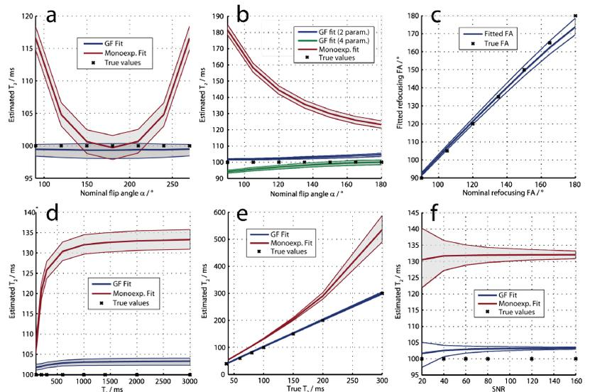
Fig 1.: Estimated median  $T_2$  values for different flip angles and slice profiles (a,b), estimated  $B_1+$  for different angles (c) and  $T_2$  for varying  $T_1$  (d),  $T_2$  (e) and SNR (f). Shaded areas are from lower to upper quartile.
