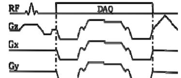
Fig.1 Gradient waveforms of a four-half-echo ME-VIPR sequence.
