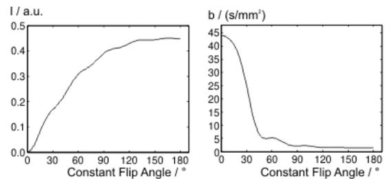
**Fig. 1:** Left: Simulated signal response measured with a typical 2D-TSE sequence depending on the constant flip angle for the representative tissue. Right: Dependence of the net b-factor on the flip angle. For low flip angles the diffusion weighting becomes more pronounced.
