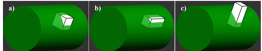
Figure 1: An anterior-posterior oriented fiber bundle is shown. The orientation of the acquisition plane is irrelevant for isotropic voxel sizes (a), but not for anisotropic voxel sizes. In (b) and (c), anisotropic voxel sizes are shown (with equal in-plane resolution and slice thickness), but in (b) the acquisition slice is perpendicular to the bundle (coronal), whereas in (c) the acquisition slice is parallel to the bundle (axial). The resulting difference in partial volume effect with the surroundings can be observed clearly.
