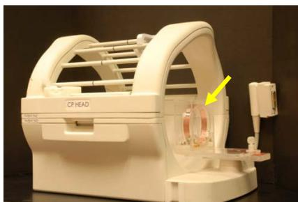
**Figure 1.** <sup>31</sup>P Birdcage Coil with <sup>1</sup>H Loop Coil indicated by arrow.
