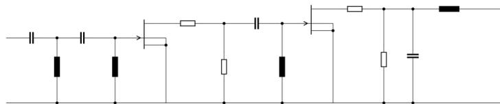
Fig 1. LNA small-signal circuit
