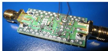
Fig 2. Picture of the PCB of the dual-stage LNA.
