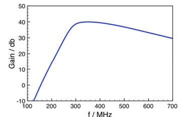
Fig 3.  $S_{21}$  of the 7 T dual-stage LNA
