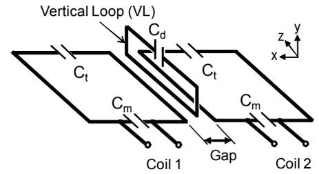
Fig. 1 Two-element coil array with vertical loop
