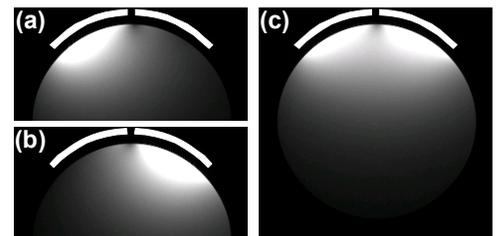
Fig. 6 Phantom images from coil 1 (a), coil 2 (b), and composition of coils 1 and 2 (c). Positions of coil elements are indicated by solid white lines.
