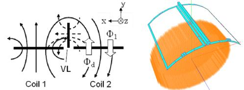
Fig. 2 Magnetic flux generated by coil 1 and VL Fig. 3 Position of coil and phantom
