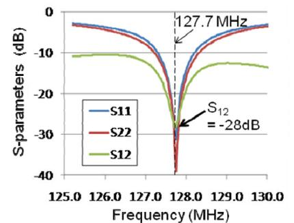
Fig. 5 Measured S-parameters of two-element coil array with VL
