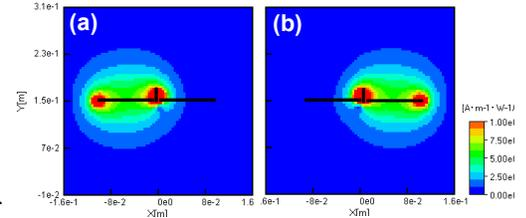
Fig. 4 Calculated axial sensitivity maps of two-element coil array with VL ((a) coil 1, (b) coil 2)
