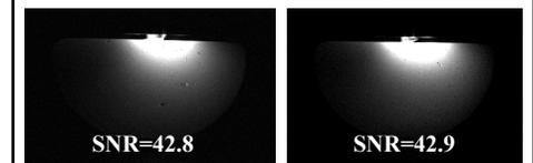
Figure 3. Spin echo images of tissue equivalent phantom; automatic matching system left, and discrete capacitors right
