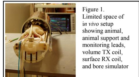
Figure 1. Limited space of *in vivo* setup showing animal, animal support and monitoring leads, volume TX coil, surface RX coil, and bore simulator
