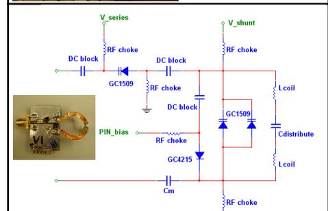
Figure 2. Schematic and picture of varactor network
