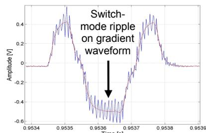
**Fig 3. The switch-mode ripple**
