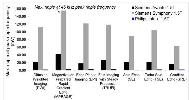
**Fig 4. The maximum ripple voltage at peak ripple frequency**
