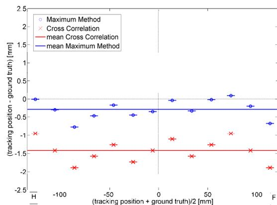
Figure 3 Bland-Altman plot of the data from the maximum and cross-correlation methods. 0 corresponds to scanner isocenter. The average result from cross-correlation was more accurate than the maximum by greater than 1 mm.
