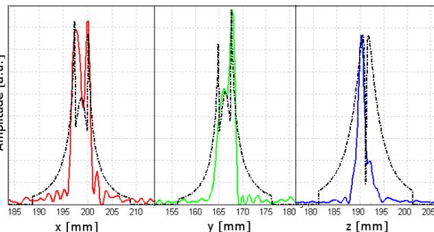
Figure 2 Signals in the spatial domain along the 3 dimensions (X, Y, and Z) and the corresponding theoretical model position (black, dotted lines) which gave the greatest cross-correlation value.
