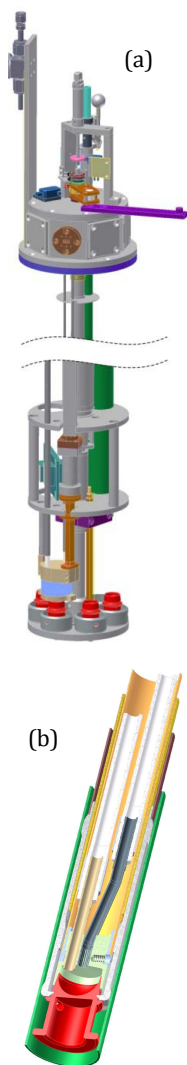
Figure 1 Design of the DNP probe (a) and the dissolution stick (b).
