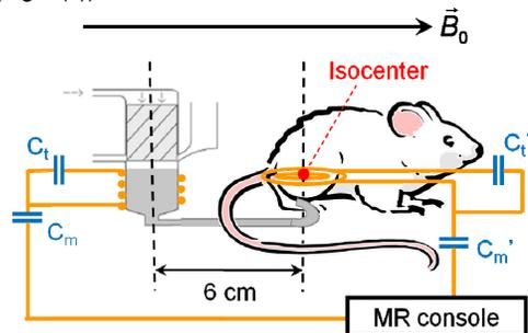
**Fig 1:** Sketch of the experimental setup inside the magnet bore. The distance between the center of the <sup>13</sup>C coil wound around the pump and the animal <sup>13</sup>C surface coil was set to 6 cm.
