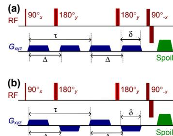
**Fig. 1: acceleration-sensitive (a) and velocity-sensitive (b) preparation modules. The motion-sensitisation gradients (MSG) are shown in blue.**
