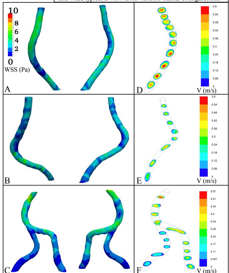
Figure 2. A-C) Time-averaged WSS distributions of Subjects 1-3, respectively (colorbar in A applies to A-C). D-F) Axial velocity contours in Subjects 1-3, respectively.
