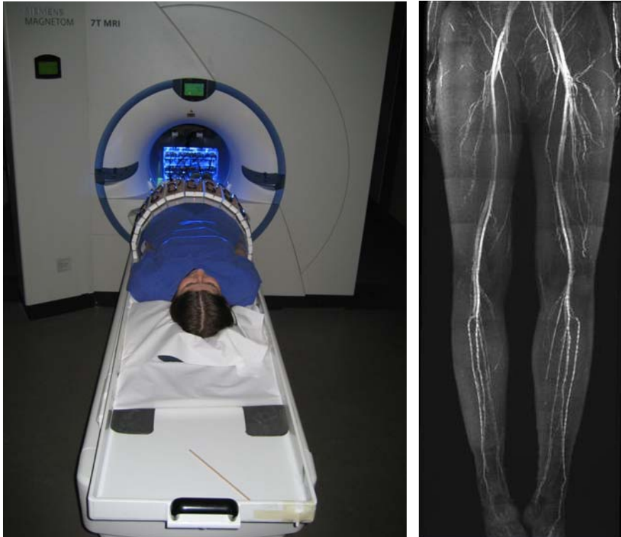
Figure 2 depicts a 16-channel transmit/receive coil based on stripline elements [17]. The coil is mounted on the patient table of the imager, and the subject can be slid through the coil from station to station on a rolling table platform (AngioSURF). This arrangement enables multistation imaging and the examination of the peripheral run-off vessels (right).
