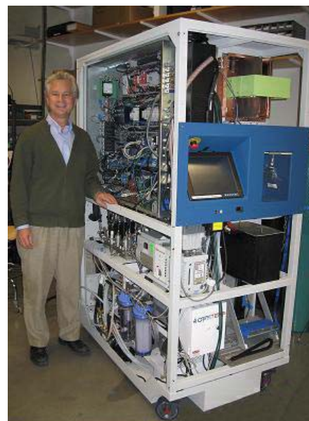
Fig.3 High production xenon polarizer incorporating this high-brightness spectrally-narrowed laser.
