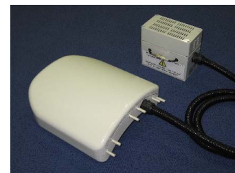
Figure 2 – 13 C/ 1 H liver coil built for in vivo human 1 H decoupled 13 C spectroscopy.
