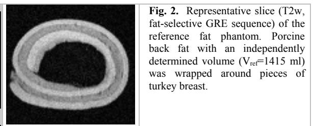
**Fig. 2.** Representative slice (T2w, fat-selective GRE sequence) of the reference fat phantom. Porcine back fat with an independently determined volume ( $V_{ref}$ =1415 ml) was wrapped around pieces of turkey breast.
