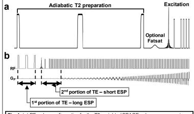
**Fig. 1.** (a) RF-pulse configuration for the T2-weighted SPACE pulse sequence using an adiabatic T2 preparation before each excitation RF pulse. (b) Allocation of the echo time between the preparation (long echo spacing [ESP]) and echo train (short ESP).
