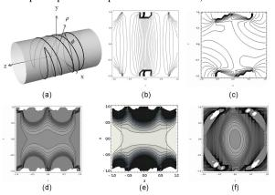
**Fig. 1:** Gz phase-gradient coil for horizontal B<sub>0</sub>. (a) coil, (b) phase plot in sagittal plane, (c) phase plot in transverse plane, (d) magnitude plot in sagittal plane, (e) magnitude plot in coronal plane, (f) magnitude plot in axial plane.
