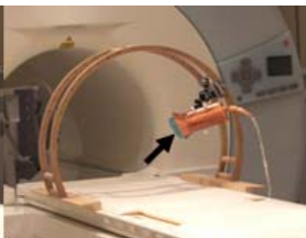
Figure 1. US transducer (EM shielded) embedded in the gel-filled bag and its holder fixed to the orbital ring
