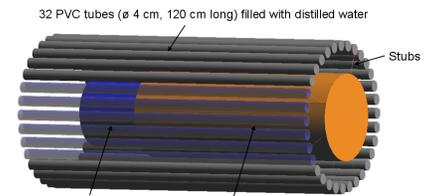
Figure 1. The set-up. Phantom contains 3 gr/l saline solution ( $\epsilon_r=80$ ,  $\text{cond}=0.3$  S/m). The coaxial waveguide is formed by the scanner's RF shield/bore ( $\phi$  58 cm) and a hollow cylindrical inner conductor ( $\phi$  32 cm). Electrical permittivity of the tubes is 80. To perform mode excitation in the coaxial waveguide 8 transverse stubs were placed around the inner conductor.
