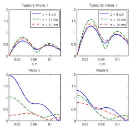
Figure 4. Simulated (top row) and measured (bottom row)  $B_1^+$  fields of the three stubs, located at  $0^\circ$ ,  $45^\circ$  and  $90^\circ$ .
