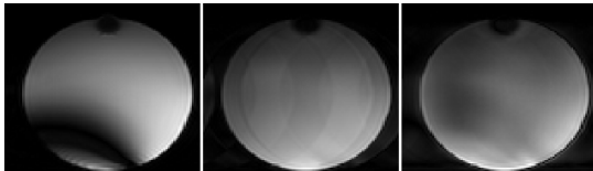
Fig. 3. a) Conventional TSE, b) adiabatic TSE without splitting the even and odd echoes, and c) the adiabatic TSE where the even and odd echoes are separated in k-space.
