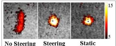
Figure 1. Representative thermal ablations without steering (top), with steering (middle) and with no motion (bottom). Motion is primarily along the vertical direction.
