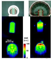
Figure 4: photographs of a) <sup>1</sup>H/<sup>23</sup>Na quadrature birdcage (TXRX,left column) and b) dual resonator system (TORO, right column) and SNR maps of a phantom filled with 100mM NaCl (middle row) and a human head (lower row).
