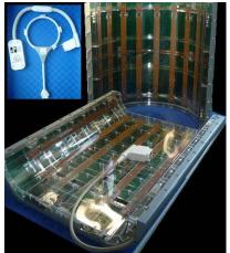
Figure 1: <sup>23</sup>Na asymmetric birdcage resonator receive-only surface coil preamplifier-holding adapter box (inset).
