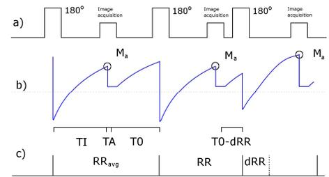
Fig. 1. Timings in a repeated IR sequence: a) RF pulses; b) longitudinal magnetisation and its values before acquisition begins – a delayed ECG trigger results in increase of  $M_a$ ; c) ECG signal – first a normal RR interval ( $RR_{avg}$ ), followed by a shorter one ( $RR=RR_{avg}-dRR$ ).
