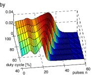
Figure 1: simulated MTR<sub>asym</sub>(1.9 ppm, 2 µT) over duty cycle and pulse number n
