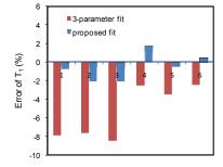
Fig. 2. Error of the  $T_1$  fitted with the proposed regression algorithm and the conventional three-parameter algorithm, using the signal intensity from IR-prepared segmented GRE sequence in Look-Locker scheme.
