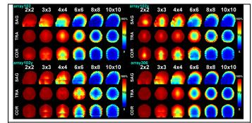
**Figure 2.** The spatial distribution of 1/g-facor in mid-sagittal, mid-coronal, and one axial slice using array102, array102x, array102y, and array306 geometries at R=2x2, 3x3, 4x4, 6x6, 8x8, and 10x10 respectively.
