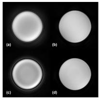
Figure 3 Phantom images acquired by UTE sequence without (a,c) and with (b,d) multiple function models. Gradient amplitudes are 4.7 mT/m (a,b) and 9.4 mT/m (c,d).
