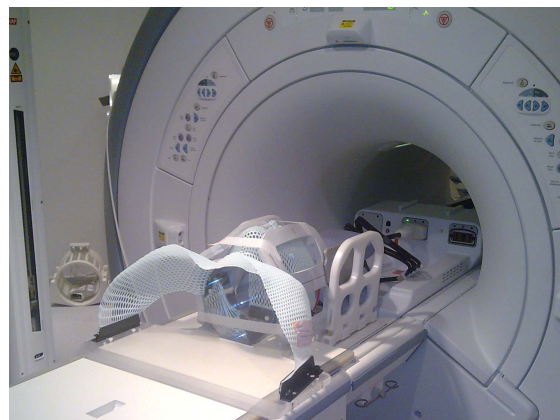
Figure 1. Surface coil positioned laterally around a thermoplastic face mask secured on a flat table
